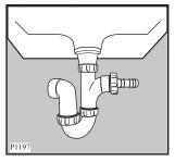
Push the drain hose onto the spigot and secure with a clip if required, ensure a loop is formed in the drain hose (see diagram) to prevent waste from the sink entering the washerdryer.
